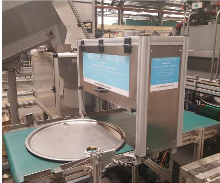
Deployed 360mm from its target, two P4-ORs with 12 and 16 mm lens respectively and white dome light inspects for defects on flanges of drum top on running conveyor
