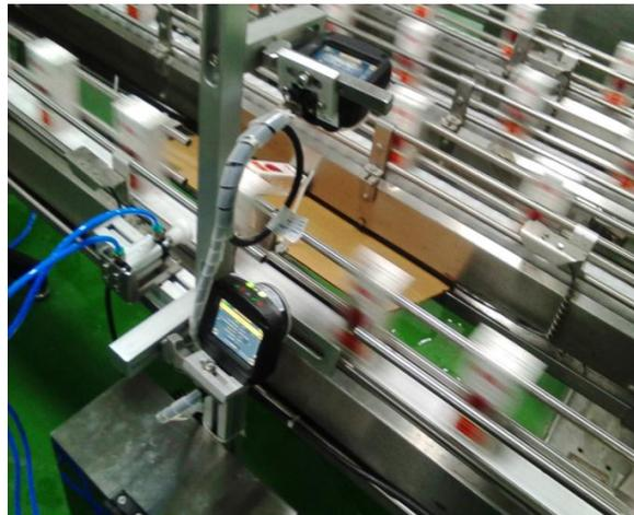
Deployed 160mm from its target, an IVu Plus TG-Gen2 with 12mm lens inspects for presence/absence detection of date code on box & Deployed 110mm from its target, an IVu Plus BCR-Gen2 with 12mm lens inspects for verification of 2D code on box.
