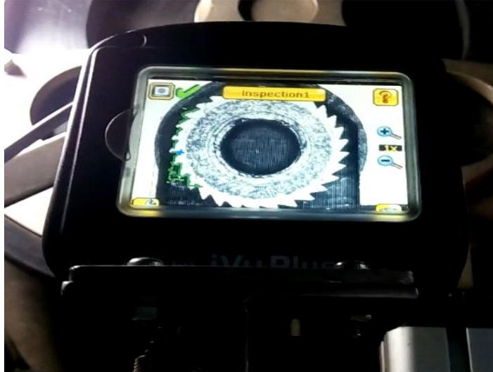
Deployed 120mm from its target, an iVu plus TG with 12mm lens inspects for verification of direction of gear teeth on rotary machine
