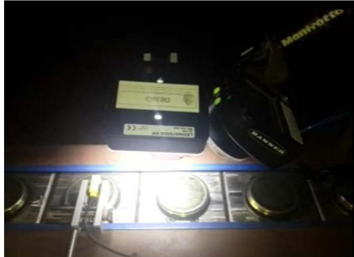
Deployed 120mm from its target, an iVu plus TG with 12mm lens inspects for the location and presence of, and twist on gasket on high speed Conveyor.
